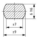
NOTE In  $\emptyset$ 6 h6,  $\emptyset$  indicates diameter, the 6 represents 6 mm, and h6 is a "class of fit" tolerance which is a sliding fit for a pin or shaft.
