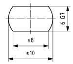
NOTE In  $\emptyset$ 6 G7,  $\emptyset$  indicates diameter, the 6 represents 6 mm, and G7 is a "class of fit" tolerance which is a sliding fit for a hole.
