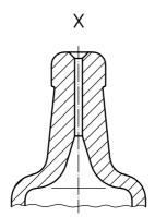
NOTE X dimension and internal shape of the bore are agreed upon between customer and manufacturer.
