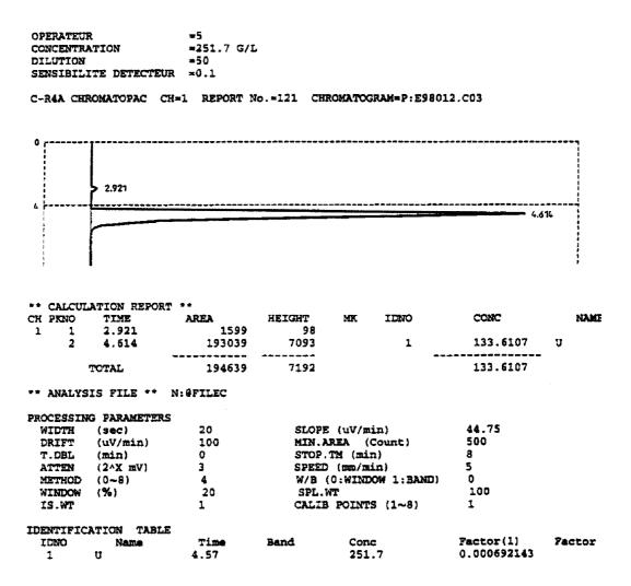
Figure A.1 — Example of a uranium concentration determination using a computer-based chromatograhy package
