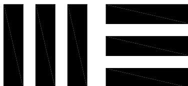
Figure 2 — Test target for checking the resolving power
