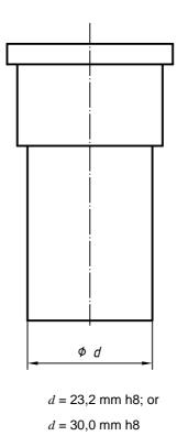
Figure 1 — Diameter of the eyepiece
