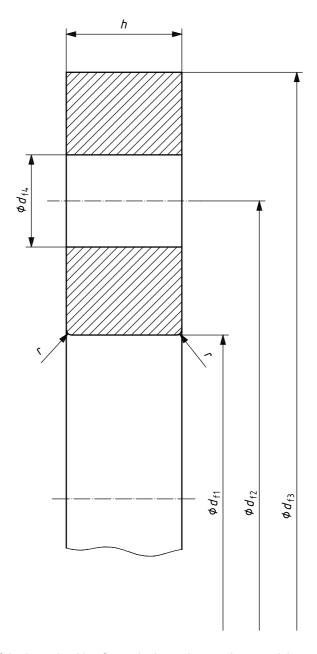
NOTE The thickness, h, of the loose backing flange is dependent on the material used.
