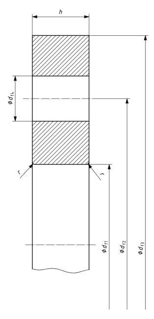
NOTE The thickness, h, of the loose backing flange is dependent on the material used.
