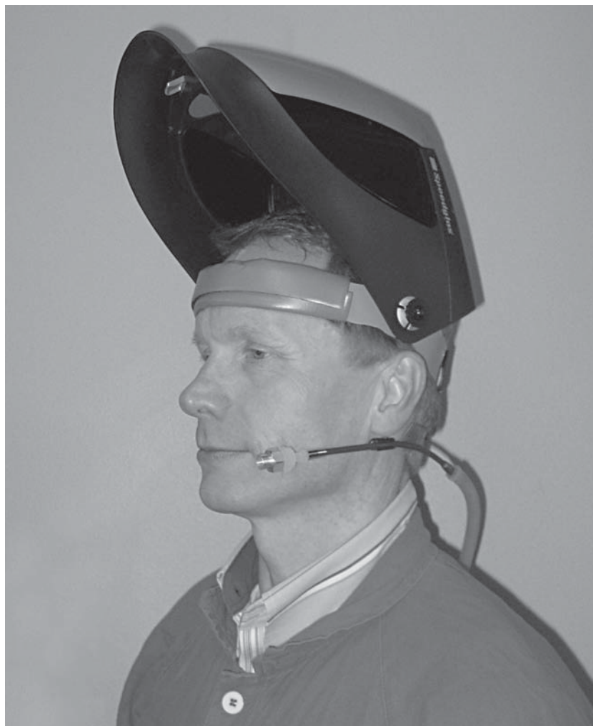
Figure B.7 — Mini-sampler on a headset beam attached to the welder's head
