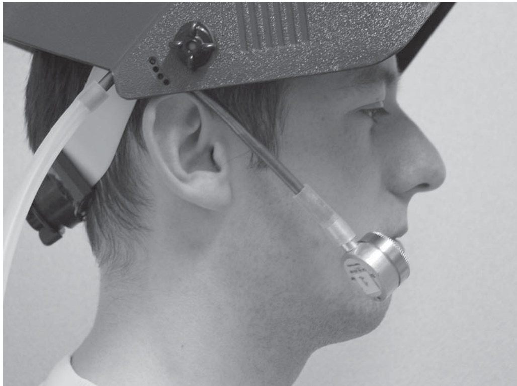
Figure B.3 — Sampler attached to the headband by means of a bent copper tube
