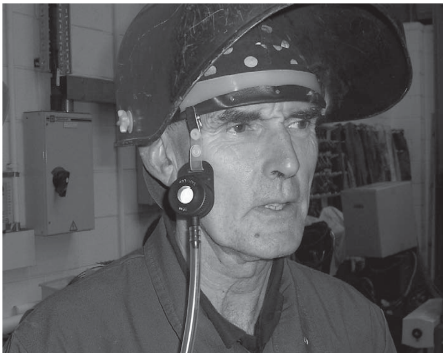
Figure B.4 — Sampler attached to the headband by means of its collar clip
