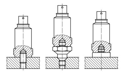
Figure 1 — Mounting methods for vibration transducers
