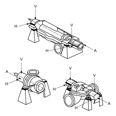
NOTE H, V (horizontal, vertical) are the two orthogonal radial measurement directions; A is the axial measurement direction.
