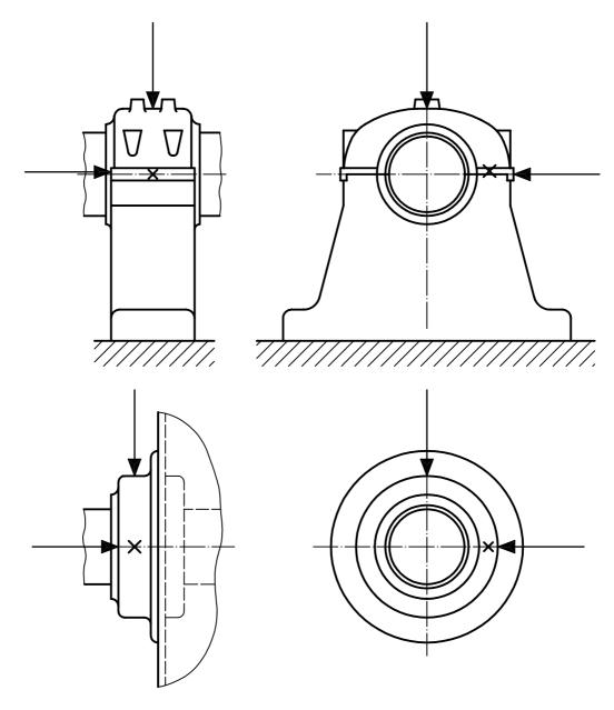
NOTE It is recommended that the location for horizontal measurements should be on the bearing pedestal and not on the bearing cap, whenever possible.
