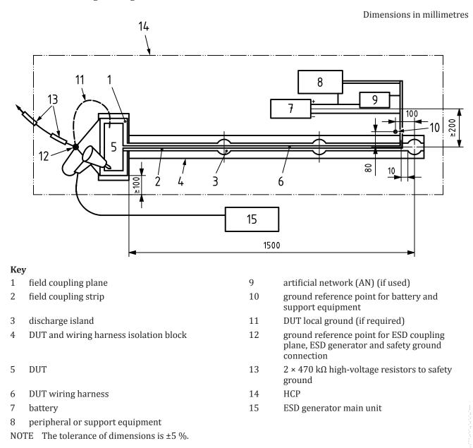
Figure F.2 — Test set-up — Application of direct discharges
