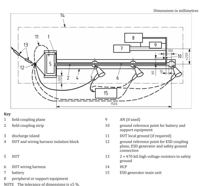
Figure F.3 — Test set-up — Application of indirect discharges
