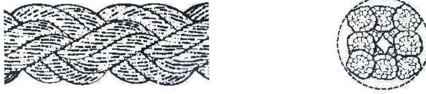
Figure 2 — Shape of an 8-strand braided rope (type L)
