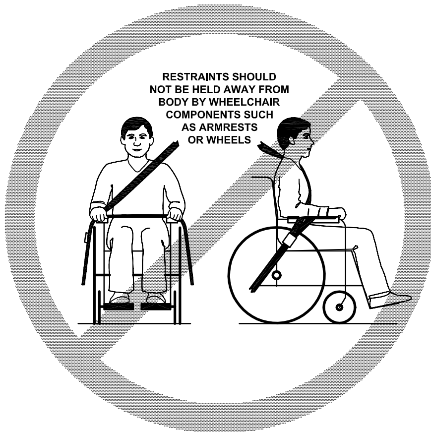
Figure 7 — Example of warning label illustrating improper positioning of occupant restraint belts
