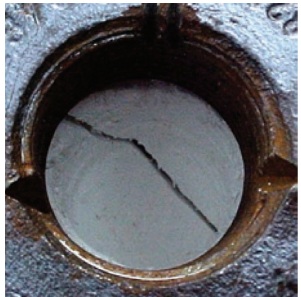
b) Crack with visible sidewalls
