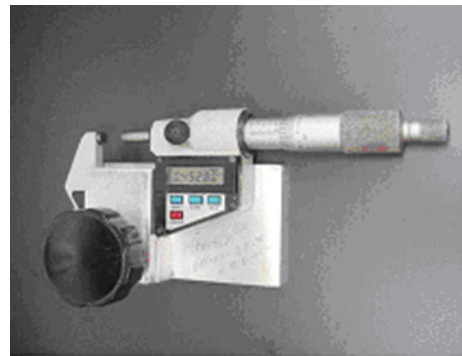
Figure 8 — Micrometer mounted to adapter
