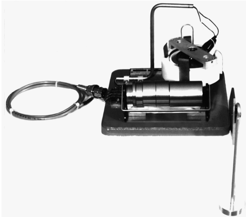
Figure 13 — Typical potentiometer calibrating device
