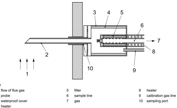
Figure 5 — Example of case where filtering material is attached at the rear stage of probe of extractive sampling system
