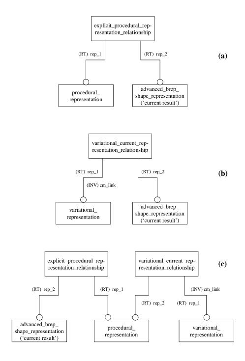
Figure E.1 – Relationships between instances of procedural, variational and explicit models for the cases of (a) no variational model, (b) no procedural model, and (c) all three models.
