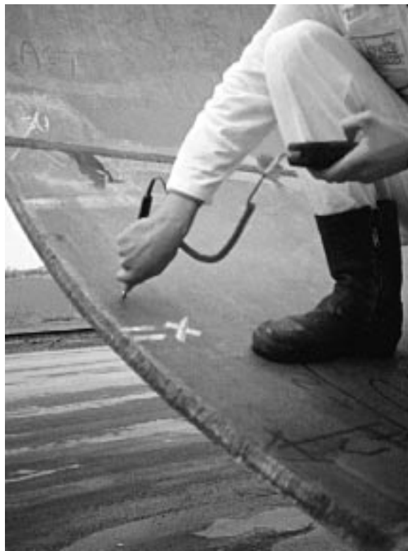
Figure 12 — Measuring shell thickness
