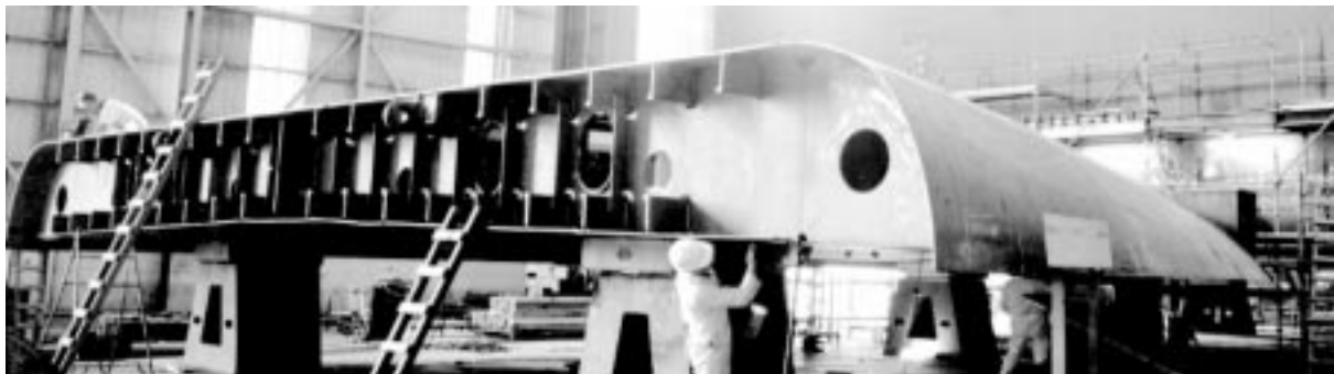
Figure 19 — Outer and inner bottom with profiles
