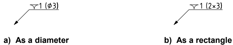
Figure 100 — Example of sink marking symbol used with maximum permissible dimension of sink mark
