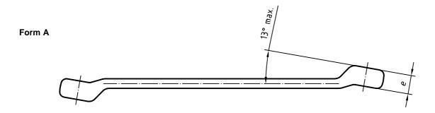
Overall dimensions of heads in accordance with ISO 3318, with the exception of the width across flat 20 mm, 23 mm, 25 mm and 28 mm.
