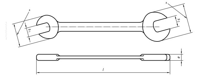
Overall dimensions of heads in accordance with ISO 3318, with the exception of the width across flat 20 mm, 23 mm, 25 mm and 28 mm.
