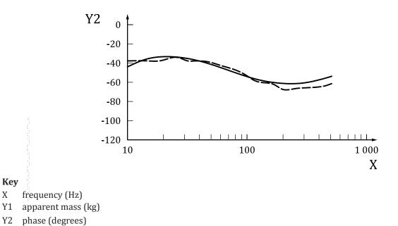
Figure B.2 — Comparison between modelled values (solid line) and mean of the synthesized values (dashed line) of the apparent mass of the human hand-arm system in the  $x_h$ -direction
