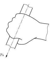
**Origin:** The centre or midpoint of the axis of the instrumented handle used for measuring biodynamic NOTE 1 response functions of the hand-arm system.
