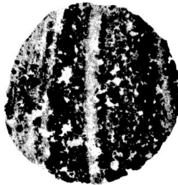
Figure 5 — Carbon or blue paper replica: not admissible because grooves are visible after sawing or grinding
