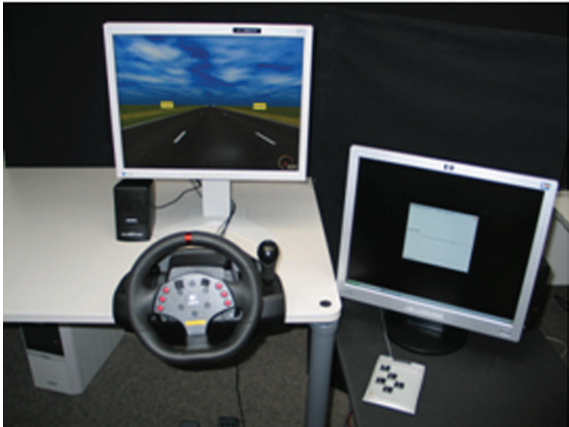
Figure A.2 — Setup for primary task (LCT example) and secondary task (CTT example)
