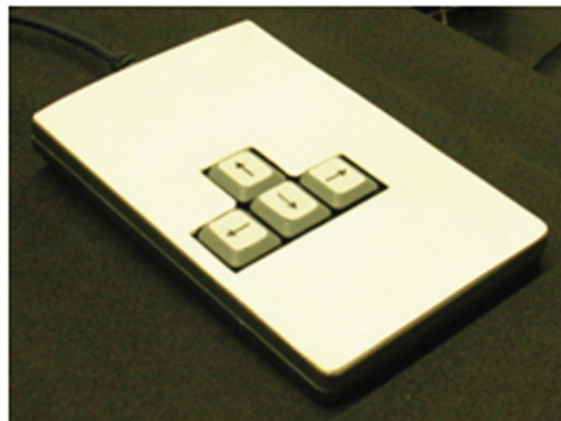
Figure 4 — Example of key-pad to move the highlight and confirm target location result
