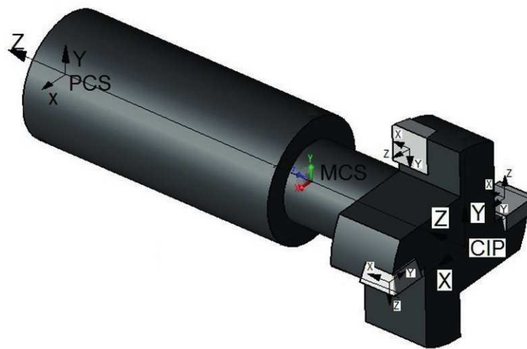
Figure 103 — Example of a data exchange model of a T-slotting end mill
