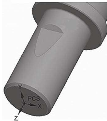
Figure 100 — Orientation of planar/clamping surfaces
