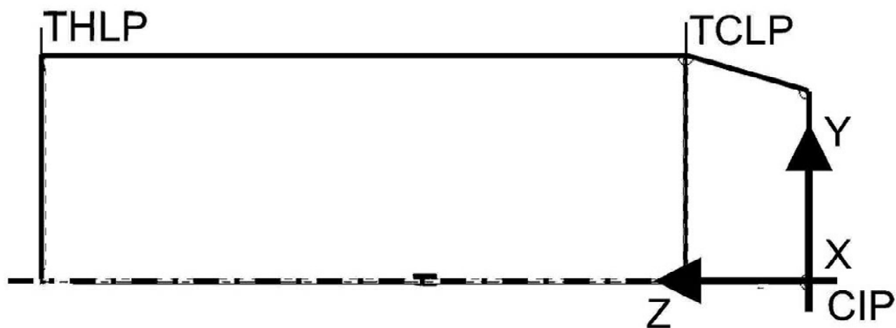
Figure 7 — Thread-cutting tap with offset shank — Sketch of cutting part
