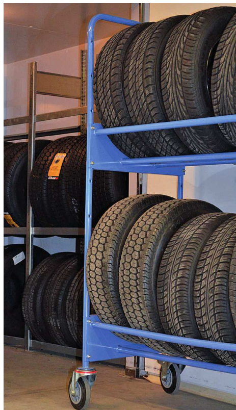
Figure B.2 — Tyre shelves with four horizontal tubes (by courtesy of M+P, The Netherlands)
