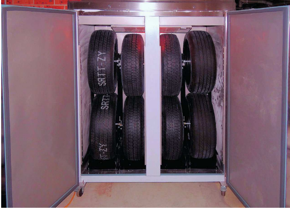
Figure B.1 — Special stand for tyre/wheel assemblies; tyres P1 and H1 stored in a refrigerator (by courtesy of Renzo Tonin & Associates, Australia)
