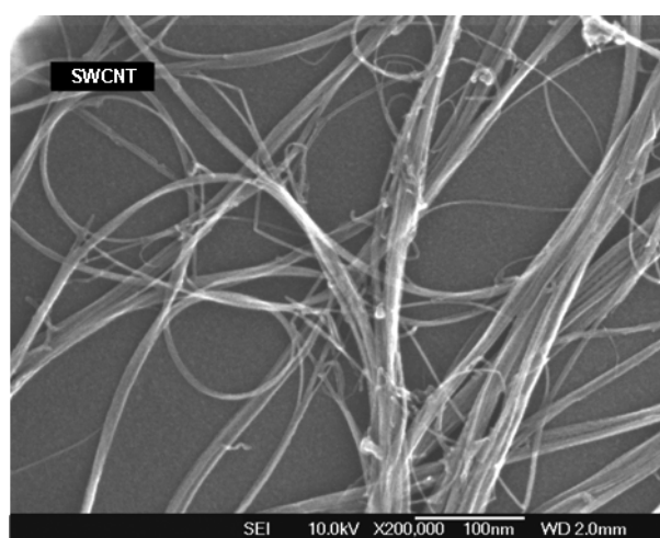
Figure D.1 — HRSEM image of SWCNT sample on a silicon wafer
