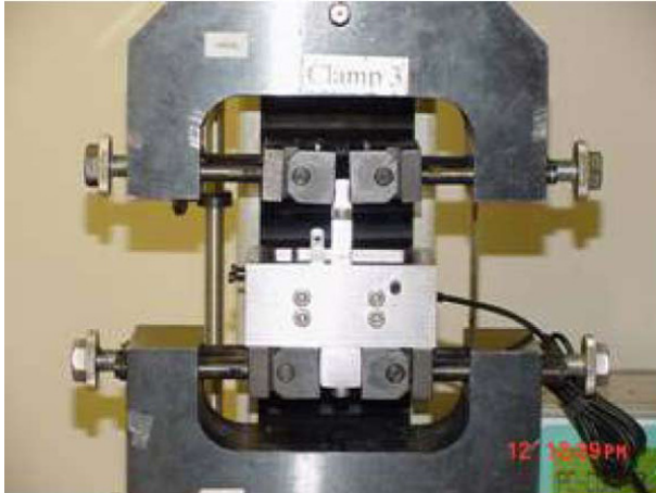
Figure D.1 — Fixture during rip-off force test
