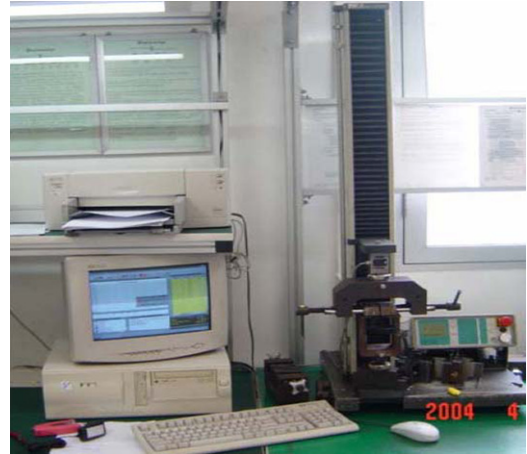
Figure D.2 — Machine for rip-off force
