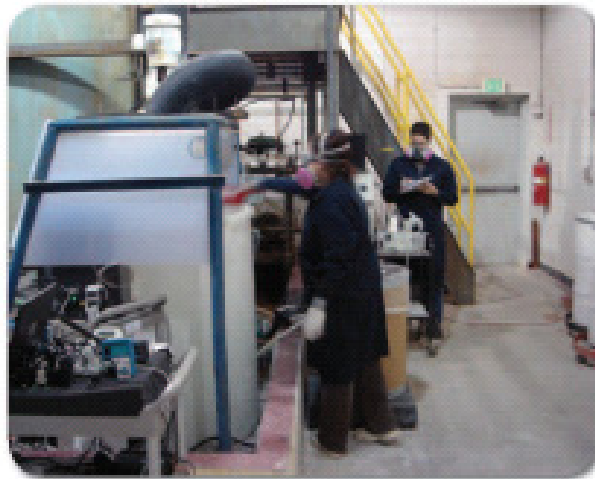
Figure 7 — Use of respirators for sampling and data collection during a mixing operation (from NIOSH Progress Toward Safe Nanotechnology in the Workplace 29 ).
