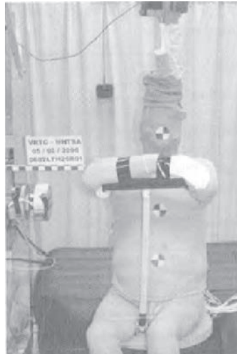
Figure C.4 — Impactor test configuration from the lateral and oblique-lateral thorax impacts conducted by OSU (front view)[49]
