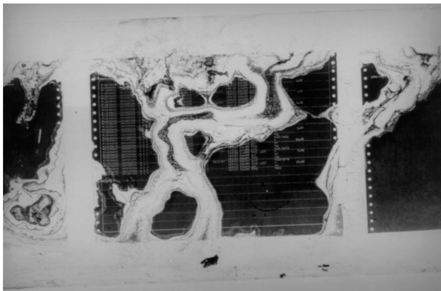
Figure C.3 — An extreme case of destruction showing the solubility of the emulsion
