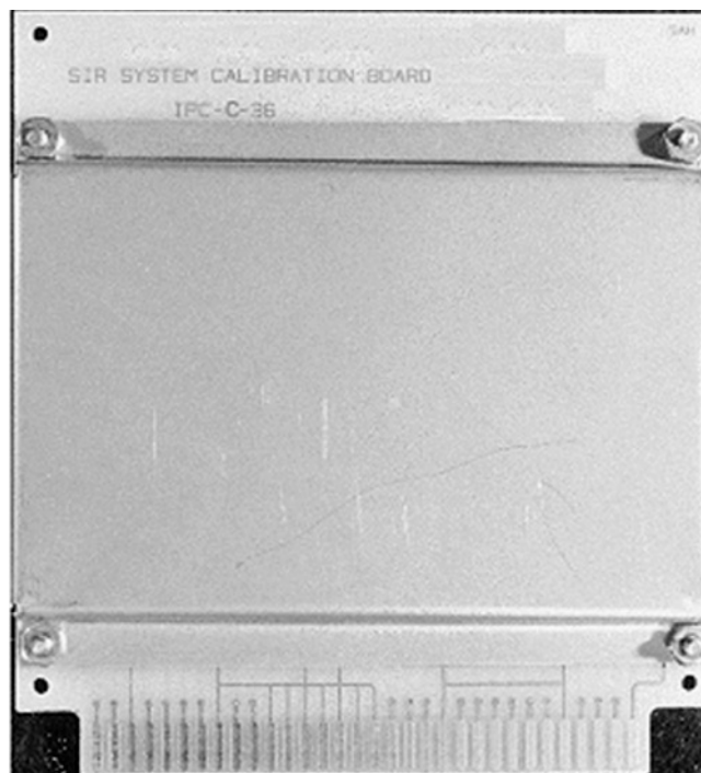
Figure 3 — Resistor verification board with protective cover
