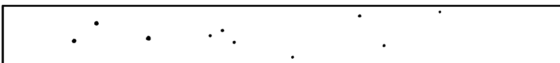
Example 8: three 1 mm, seven 0,5 mm discontinuities (scattered)
