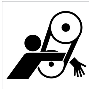
Figure A.29 — Hand and arm entanglement — Chain or toothed belt drive
