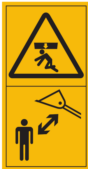
Figure C.2 — Crushing of whole body — Stay safe distance from raised loader lift arm and bucket
