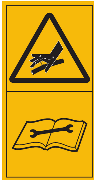
Figure C.17 — High pressure fluid — Avoid fluid escaping under pressure — Read technical manual for proper service procedures
