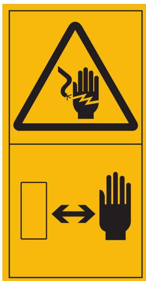
Figure C.15 — Electrical shock or electrocution — Keep hands safe distance from electrical power source
