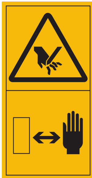
Figure C.21 — Severing of fingers or hand — Keep hands safe distance from hazard
