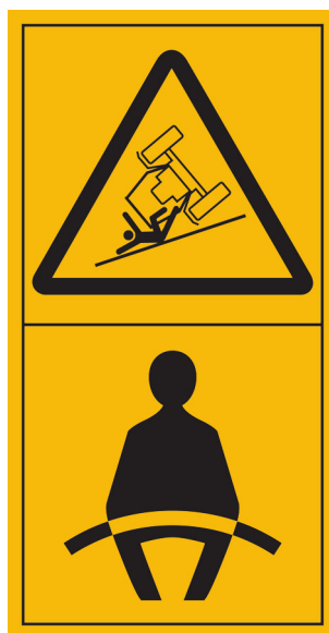
Figure C.31 — Crushing hazard due to machine rollover — Wear seat belt
