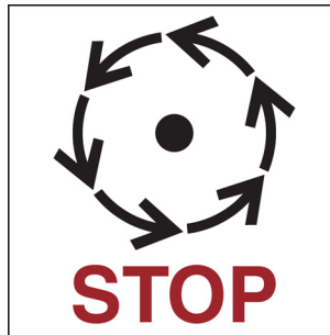
Figure B.12 — Wait until all machine components have completely stopped before touching them
