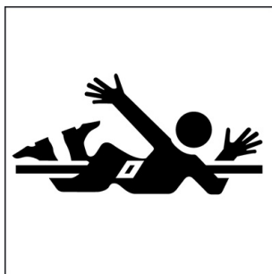
Figure A.34 — Leg or foot entanglement — Auger
