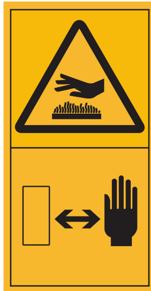
Figure C.16 — Hot surface — Burn to finger or hand — Keep hands safe distance from hazard
