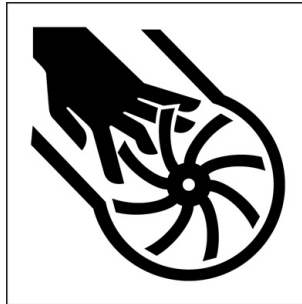
Figure A.23 — Severing of fingers or hand — Impeller blade
