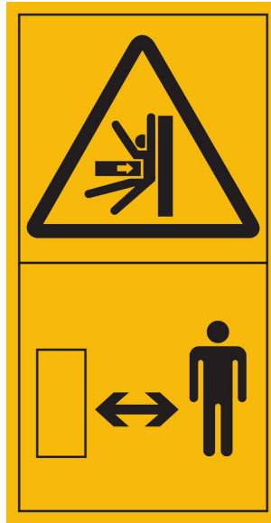
Figure C.4 — Crushing or pinning of whole body — Stay safe distance from hazard
