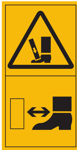
Figure C.28 — Crushing of feet — Keep feet safe distance from hazard
