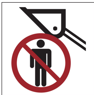
Figure B.16 — Do not reach into crushing area
