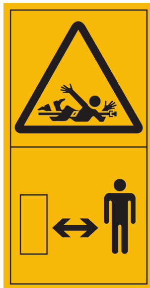
Figure C.26 — Whole body entanglement in machinery — Stay safe distance from hazard
