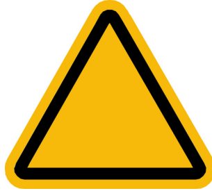
Figure 8 — Safety shape for warning signs
