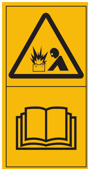
Figure C.18 — Explosion of battery — Read operator's manual
