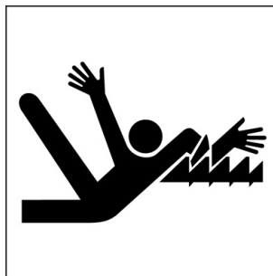
Figure A.31 — Hand and arm entanglement — Rotating gears
