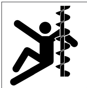
Figure A.33 — Hand and arm entanglement — Auger
