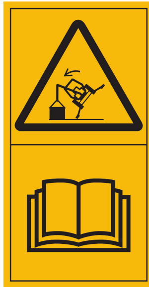
Figure C.32 — Machine tip-over or overload — Read operator's manual
