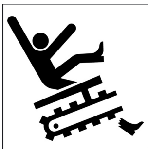
Figure A.35 — Full body entanglement — Machinery
