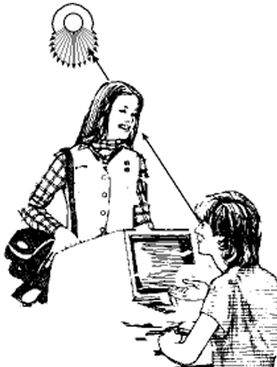
Figure A.1 — Situation under which specific measures for glare guarding are needed
