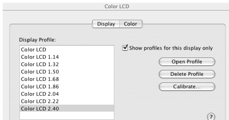
Figure D.8 — Eight gamma values that produce eight different input–output profiles for computer display
