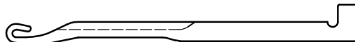
Figure 19 — Compound needle with grooved stem Figure 19 — Aiguille «compound» à gorge Bild 19 — Rinnen-Schiebernadel
