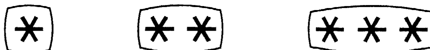
Figure 8 — Identification symbols for frozen food storage compartments (or cabinets) (for further details, see figure 17)
