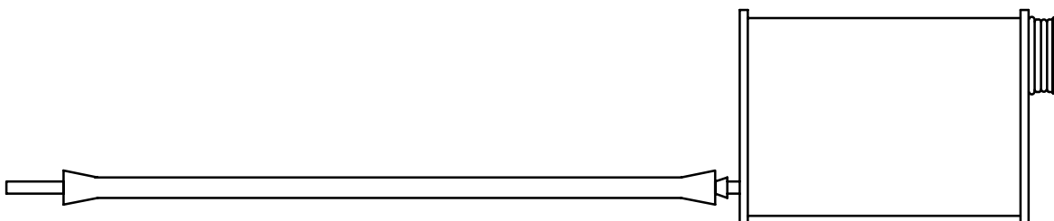
Figure 5 — Test assembly storage position
