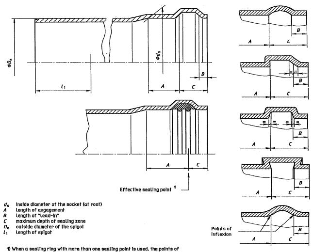
measurement for  ${\cal A}$  and  ${\cal C}$  shall be indicated by the manufacturer and these points shall give a full sealing action.
