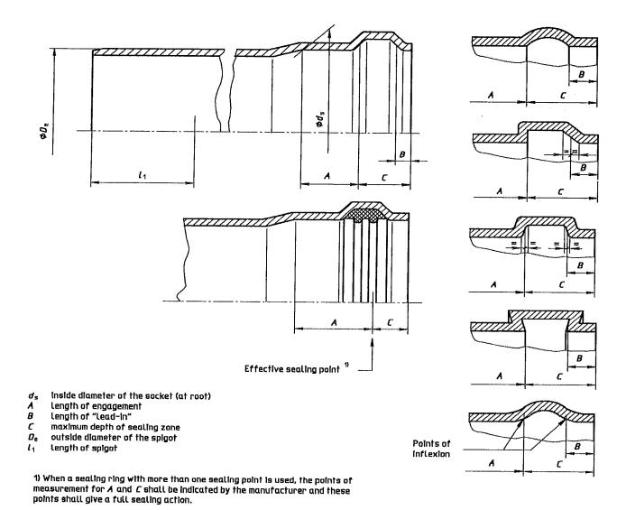
Figure 1 — Location of points of measurement for sockets and spigots
