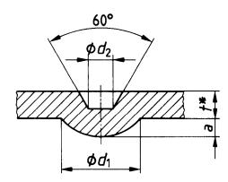
\* See annex A for relationship between sheet thickness, t, and projection diameter,  $d_1$ .
