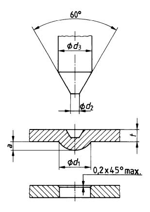
NOTE  $- \oplus d_3 > \oplus d_1$ ; for other dimensions, see table 1. All unspecified dimensions to be produced within the relevant tolerances in accordance with ISO 286-1.
