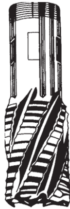
Figure C.3 — Chip-breaking mill cutter
