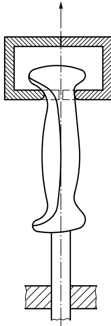
Figure 4 — Test arrangement for pulling-off force
