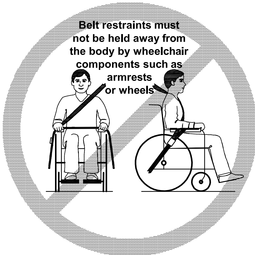
Figure 6 — Illustration of improper belt-restraint fit
