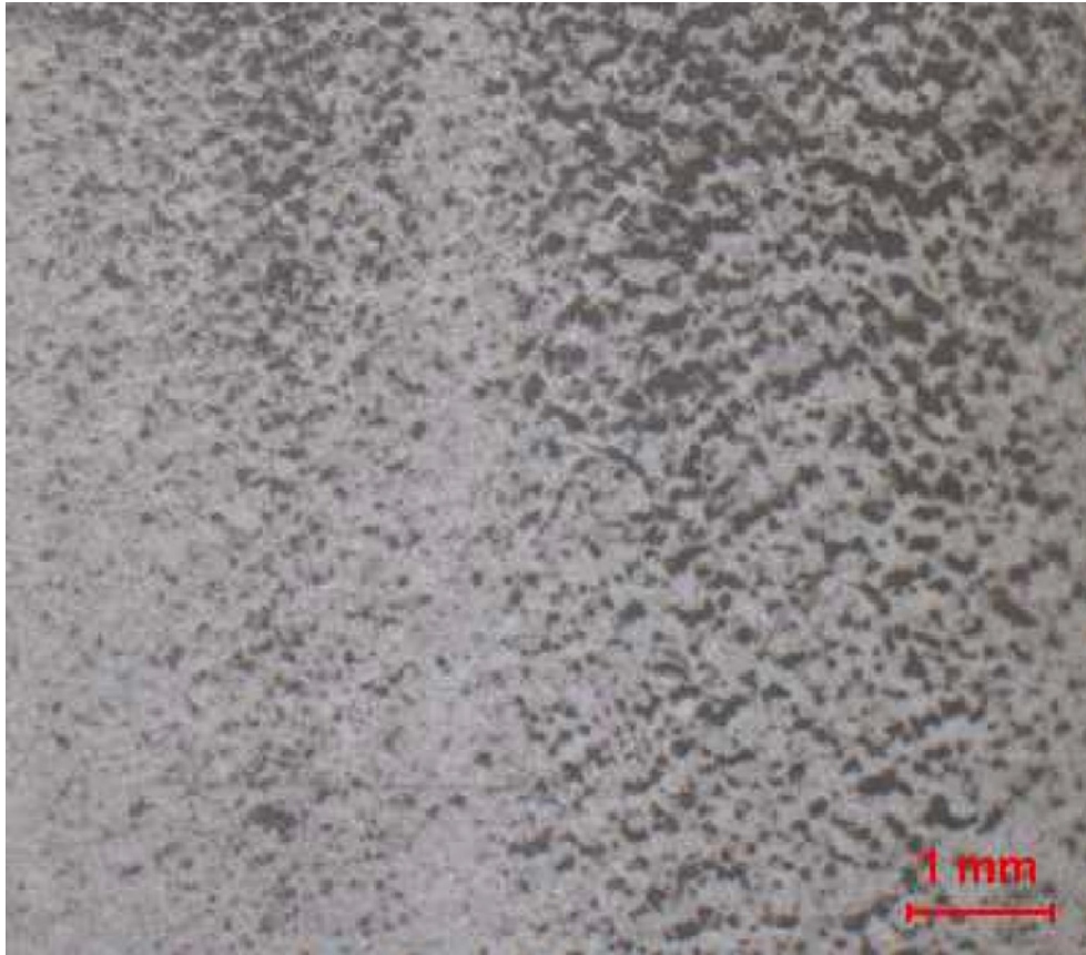
Figure 42 — Deposit of oil carbon on galvanic surface
