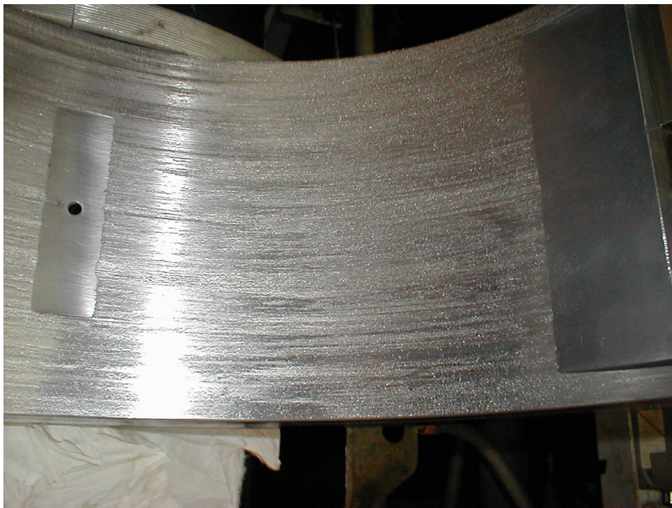
Figure 46 — Formation of electric arc craters
