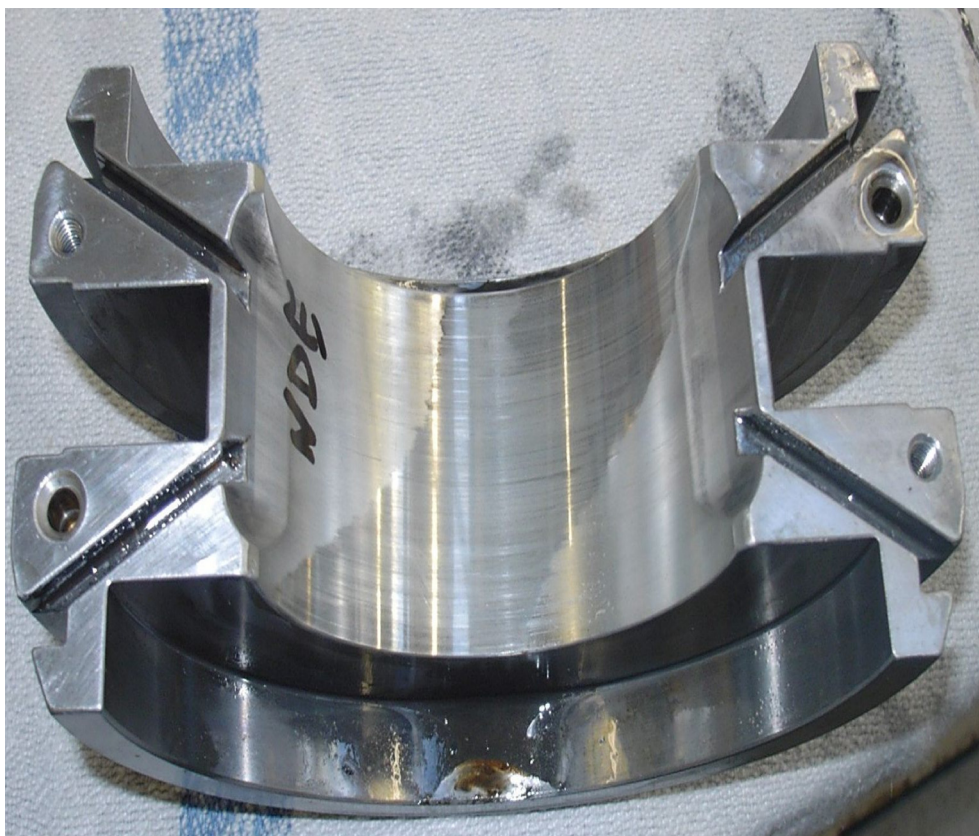
Figure 17 — Wear by misalignment between bearing backing and shaft (material: steel/tin-based white metal)
