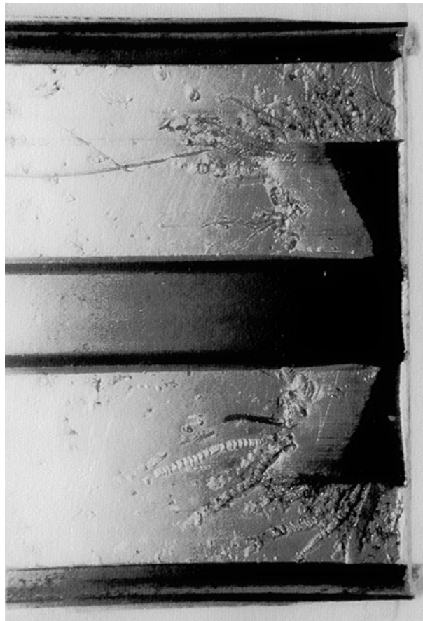
Figure 34 — Particle-migration tracks concentrated to the pocket area of a thin-walled bearing (material: steel/AlSn)
