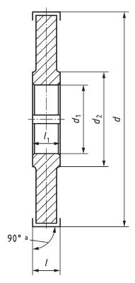
The value of 90° is the nominal cutting edge angle of the insert.
