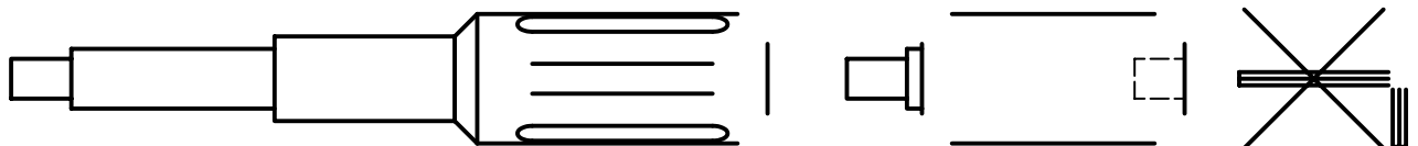
Figure B.5 — Class E: screwdriver, fixed adjustment
