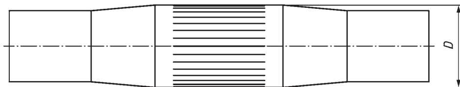
Figure 1 — External diameter of the handlebar
