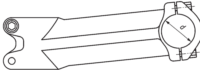
Figure 2 — Internal diameter of the stem clamp
